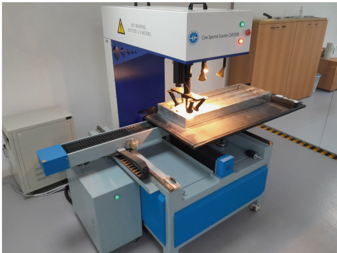
Figure 2. The drill core box is placed on the table for scanning, moving in X and Y directions. The size and technical specifications of the drill core box are entered into the controlling software. Based on these parameters, the scanner automatically does the scanning. As part of the quality control standards, each box is scanned before use.
