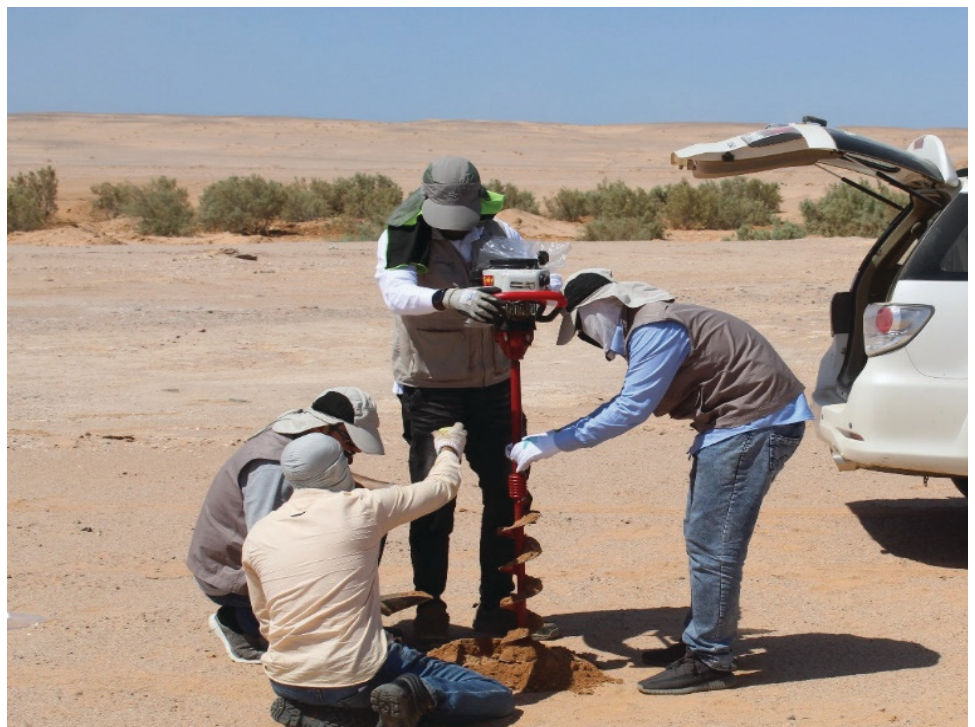
Figure 2. Auger is a device used to drill soil deposits to obtain shallow subsurface samples, NEOM Project.
