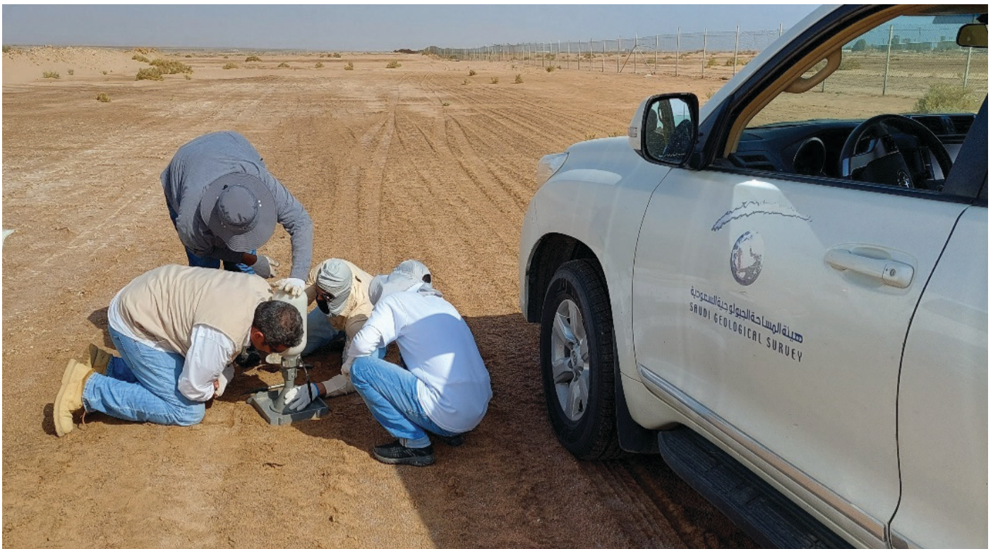
Figure 1. Photo showing the engineering geological team conducting a field density (FD) test at one of the sites, the NEOM Project.
